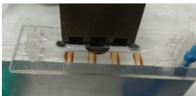
Fig. 2 Captured 1 mg of SMB in phosphate buffer in rhombic chamber chip (120 \mu L volume, 6 cm long) using special electromagnet.
